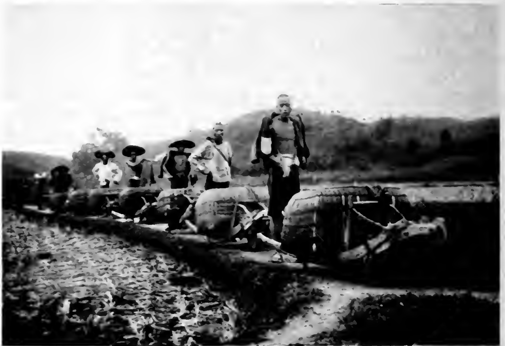
A wheelbarrow freight-train of Hunan Province, where a little kangaroo-like front wheel is useful in clearing obstacles, pauses for a breathing-spell along the great overland trail from the Yang Tze to Canton
